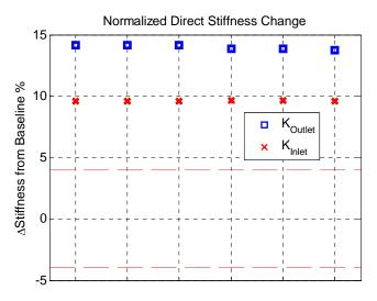
Figure 9 Direct Stiffness Verification - Over Pressurized Meter
