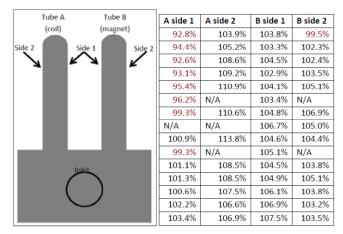
Figure 7. Tube Thinning Measurements
