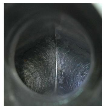
Figure 6. Eroded Inlet Manifold
