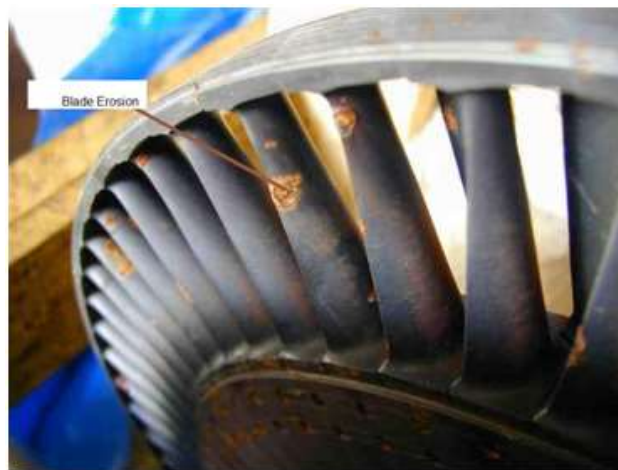
Figure 1. Water Impingement on Turbine Blades
