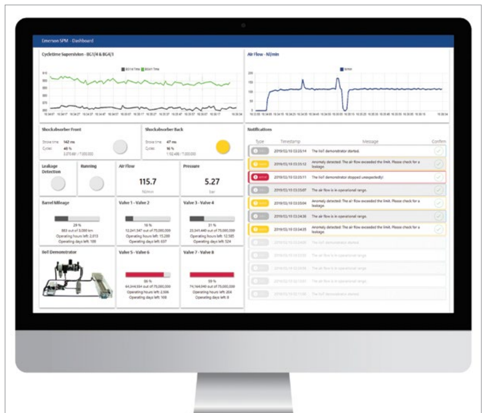
Figure 2: Operators can view pneumatics data and valuable insights on an easy-to-read local dashboard, making it simple to quickly respond to issues if they arise. (image courtesy of Emerson)
