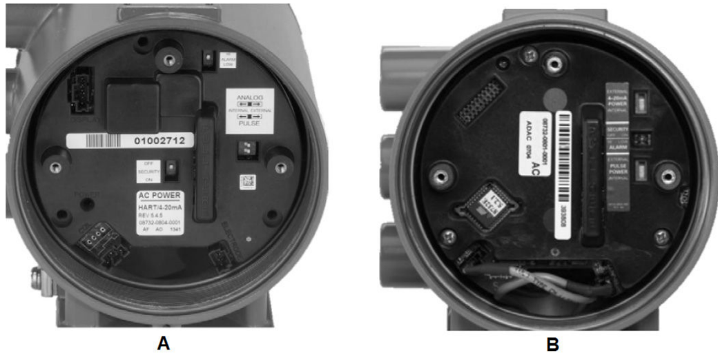
Figure 11-2: Electronics Stack Identification
