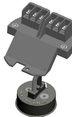
Figure 12-4: Remote Mount Socket Module
