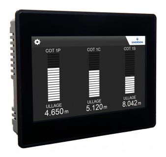
The Rosemount PDF 52 is the Graphical Display Application for the PDU 51 Panel Display Unit. It offers you an additional display unit dedicated to specific cargo tank measurements, such as the level or pressure readings with graphics.
