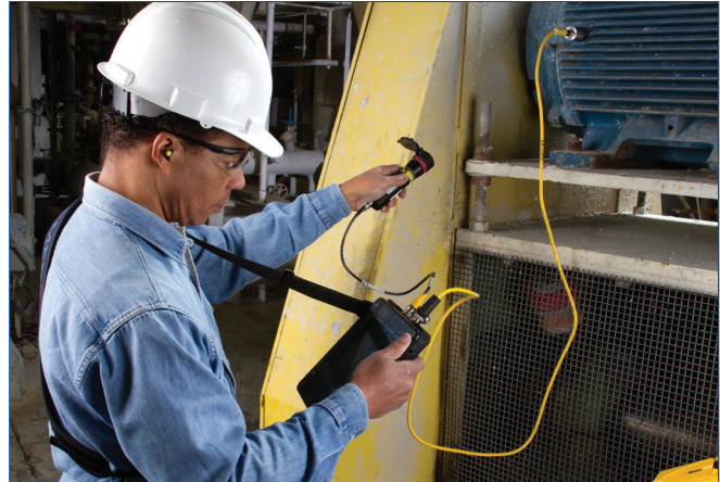
The AMS 430 Laser Speed Sensor determines shaft speed without shutting down the machine - even in extremely tight locations.
