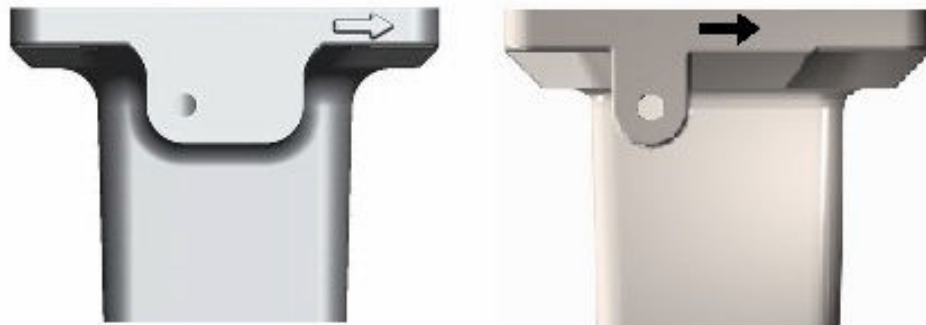
Figure 3-2: Flow direction arrow
