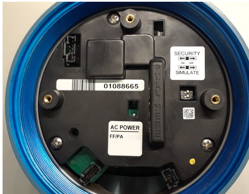
Figure 6-1: Electronics Stack and Hardware Switches
