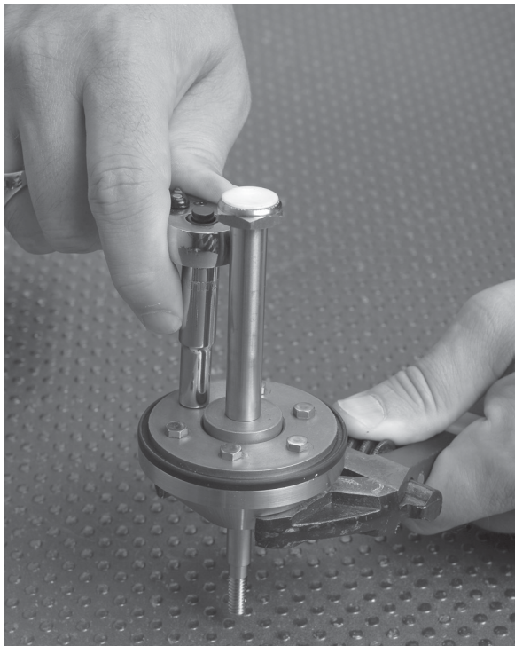
Figure 5. Use tool provided or Spring Seat (key 4) and Stem Assembly (key 2) to align Disc Retainer (key 8)
