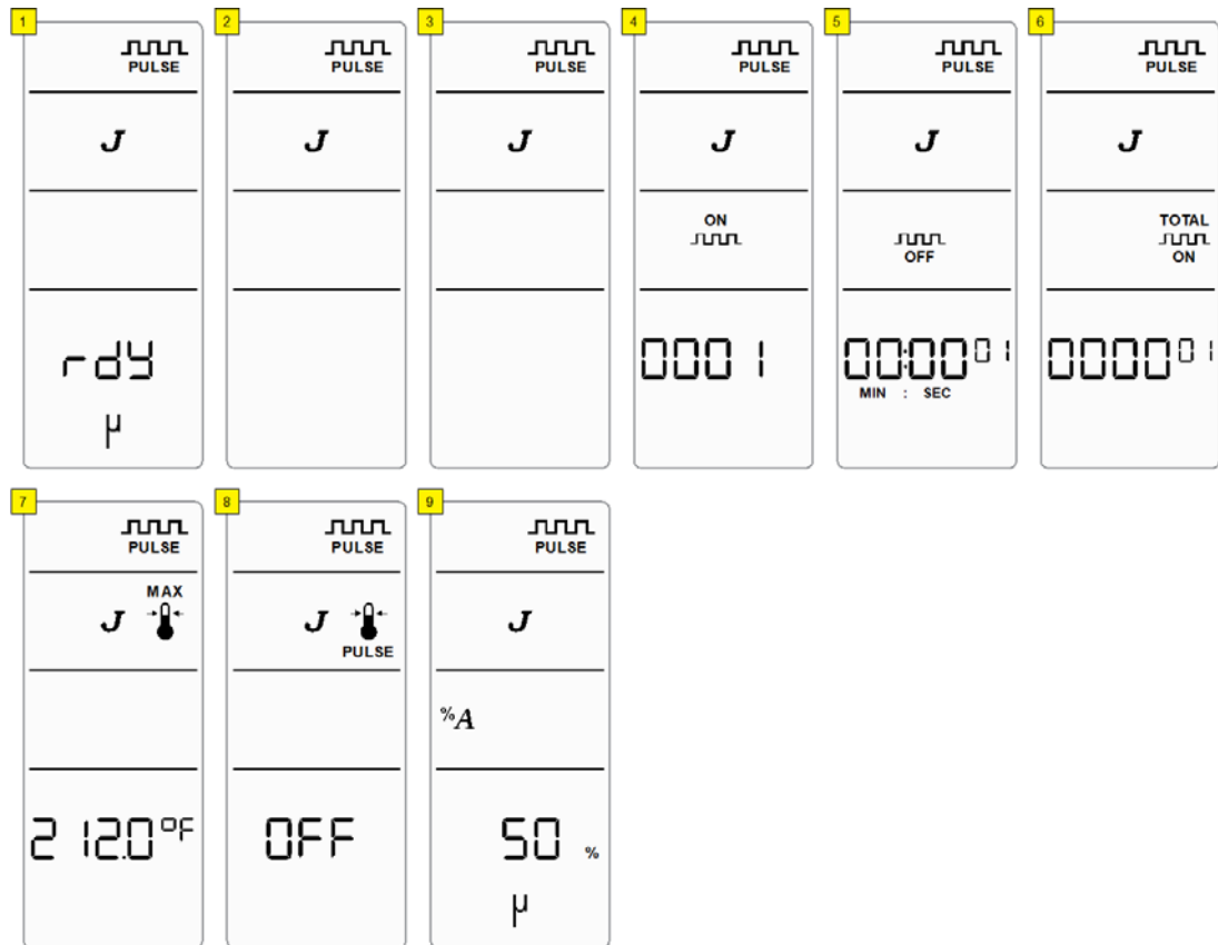
Figure 6.16 Temperature Limit - Pulsed Sonics (Energy) Mode
