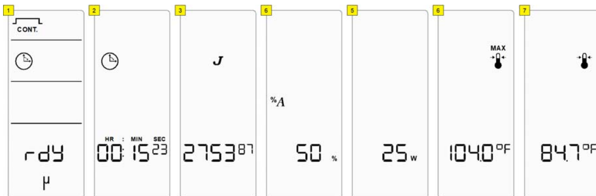
Figure 6.2 Results for Continuous Sonics - Time Mode (Example)
