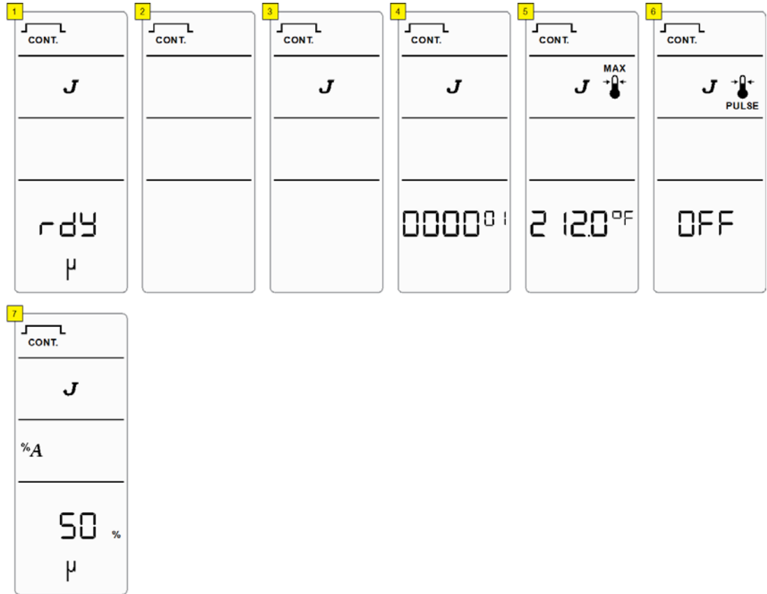
Figure 6.14 Temperature Limit - Continuous Sonics (Energy) Mode
