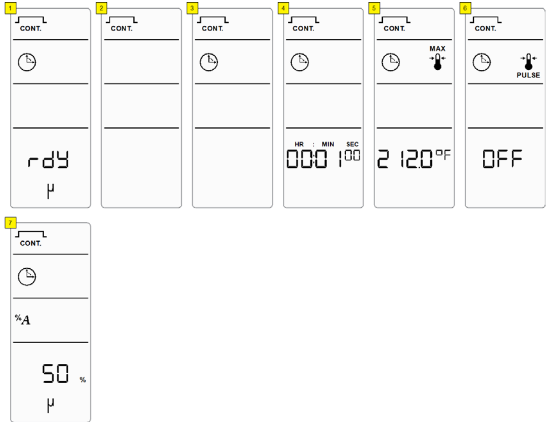
Figure 6.13 Temperature Limit - Continuous Sonics (Time) Mode
