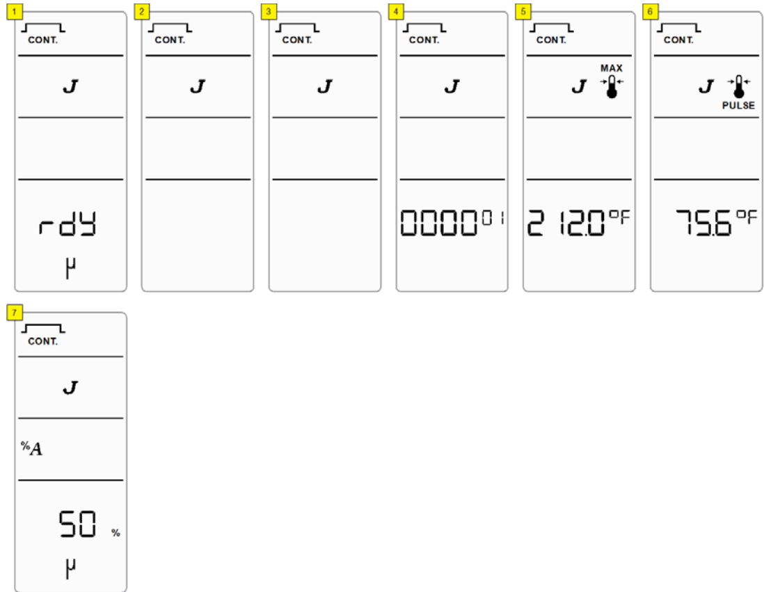
Figure 6.18 Pulse Temperature - Continuous Sonics (Energy) Mode
