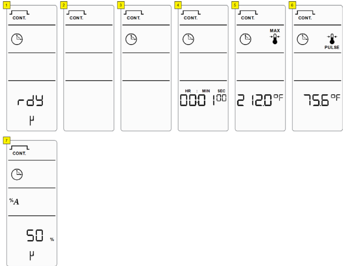
Figure 6.17 Pulse Temperature - Continuous Sonics (Time) Mode
