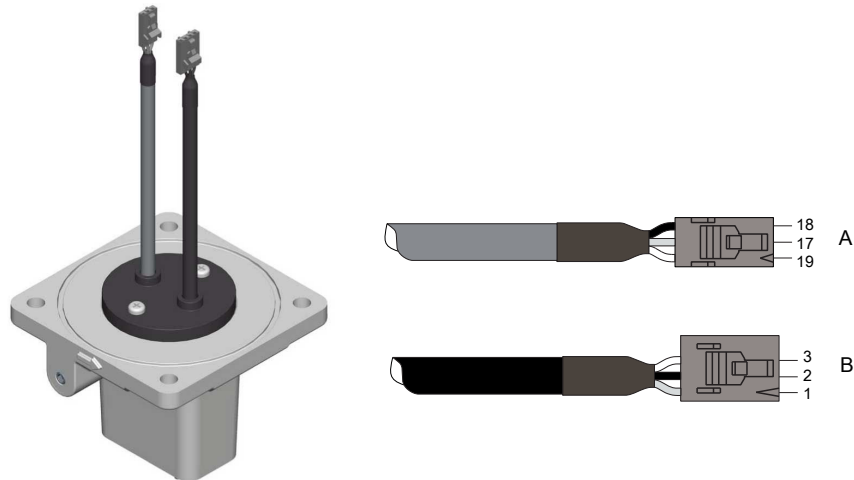
Figure 12-3: Sensor adapter direct lead pins
