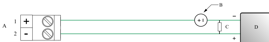
Figure 3-8: Channel A mA/HART output wiring (externally powered)
