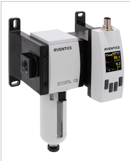
Figure 3: Much more than a flow meter, the AVENTICS™ AF2 Flow Sensor continuously monitors compressed airflow, measures 8 performance parameters, including energy, and helps detect leaks in pneumatic systems. (Image courtesy of Emerson)
