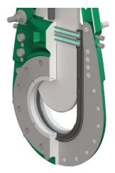
Deploy a patented gate edge seal that creates a continuous seal around the gate, together with a precision-molded elastomer seat to deliver zero leakage. This heavy-duty replaceable seat increases the contact area and resilient sealing ability of the valve compared to standard O-ring designs, resulting in superior isolation performance over an extended lifecycle.
