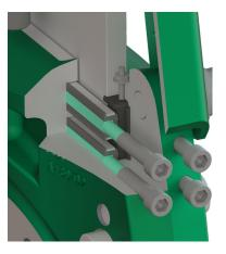
Minimize valve repair downtime with external packing adjustments that dynamically self-adjust pressure to the gate edge seal system. Repairs can be performed rapidly using standard tools and readily available spare parts. The valve is also designed to MSS-SP-135 face-to-face dimensions for simple changeout and upgrade of your underperforming valves.
