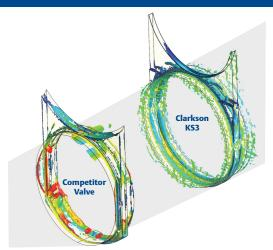
Run your processes for longer with a valve design optimized to thrive in heavy slurry conditions. A full round port eliminates protrusions into the flow, minimizing turbulence across the valve to extend body life. This not only ensures the longevity of sealing components, but also minimizes the damaging impacts of slurry on downstream pipeline equipment.
