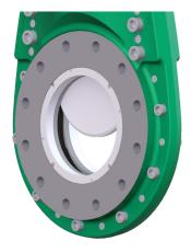
Extend the life of your valves with standard inlet and outlet hardened wear rings to protect the sealing elements and body from abrasive slurry. These durable Ni-Resist rings can be rotated 3 times through 4 positions to extend valve life and replacement intervals, allowing you to improve your asset utilization and process productivity.
