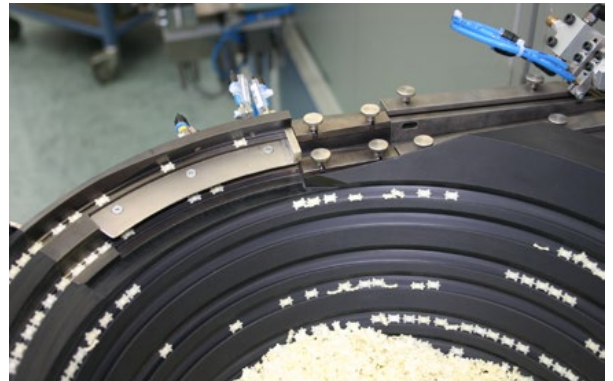
The system feeds 7 fuse variants.
