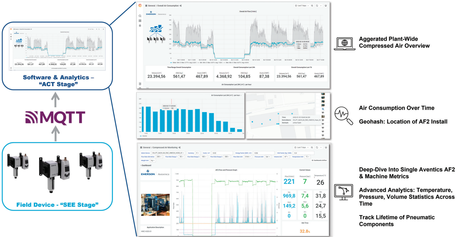
FIGURE 3: This dashboard for pneumatics applications offers a picture of a facility’s pneumatic system performance in one screen, enabling quick, informed decision-making that makes predictive maintenance possible. Courtesy Emerson
