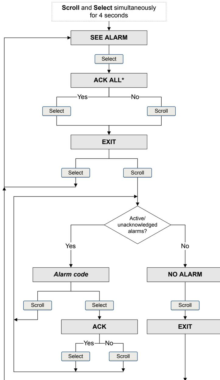
*This screen is displayed only if the ACK ALL function is enabled and there are unacknowledged alarms.*
