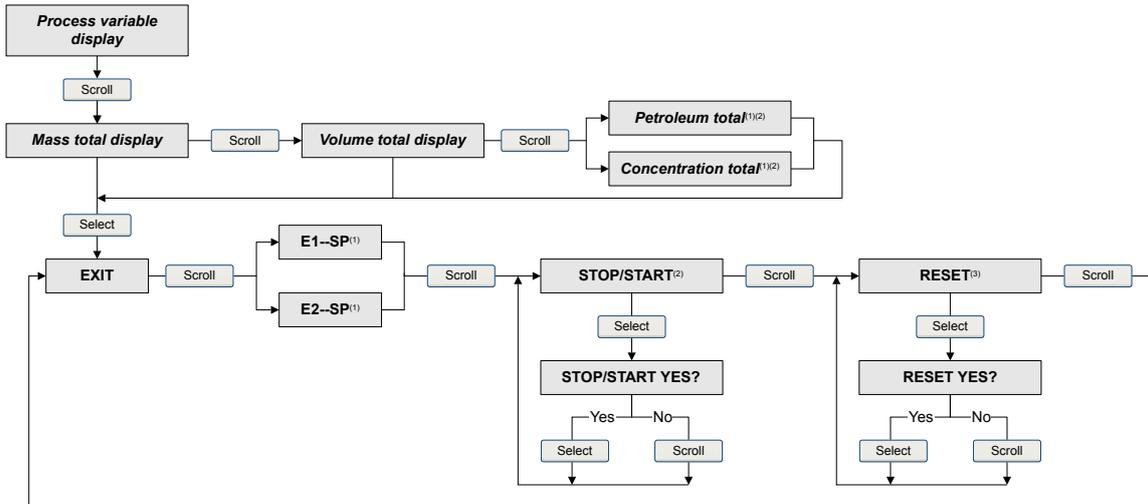
\*The Event Setpoint screens can be used to define or change the setpoint for Event 1 or Event 2 in the basic event model. These screens are displayed only if the event is defined on mass total or volume total. Note that this functionality does not apply to discrete events (the enhanced event model).
