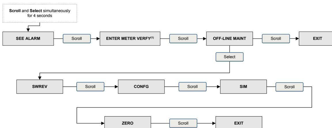
(1) This option is displayed only if the transmitter is connected to an enhanced core processor and the meter verification software is installed on the transmitter.
