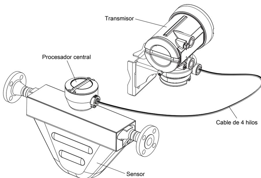
**Figura F-4: Instalación remota de 4 hilos – alojamiento de acero inoxidable**
