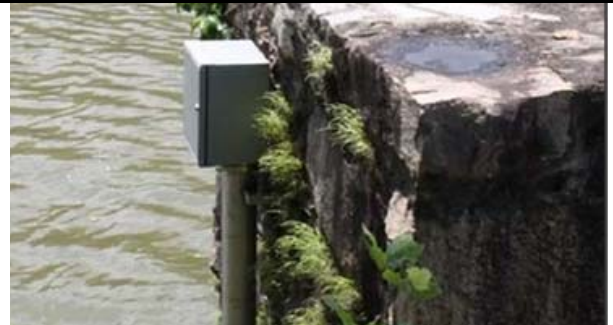
Rosemount 1199 Submersible Seal used for river level measurement
