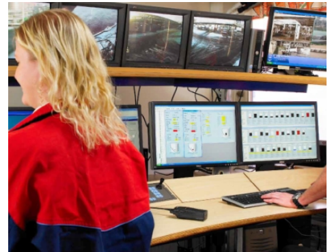
The TankMaster inventory management software is used for net volume calculations, batch transfers, reporting, alarm handling, commissioning and service.
