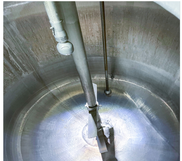
Mixing tank with multi-layer agitator blades.
