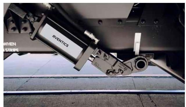
Railcar cylinder with lightweight fiberglass tube used to operate the bottom discharge doors.
