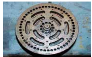
Changing oil formulation eliminated oil varnish problem and premature overhauls
