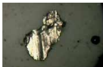
Gear tooth chunks
