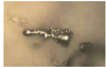
Partially melted particle from abnormal BLW
