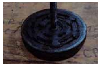
Varnish formation due to oil degradation
