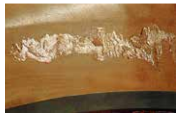
Fatigue pitting on bearing surface
