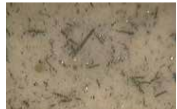
Oxidized needles from gear tooth fatigue & abnormal boundary lubewear
