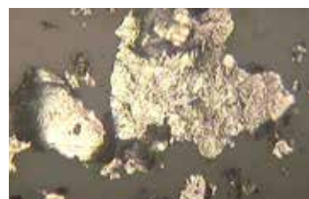
Ribbon from abrasive wear
