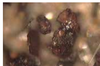
Rust from water contamination
