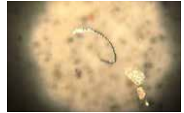
Ribbon from abrasive wear
