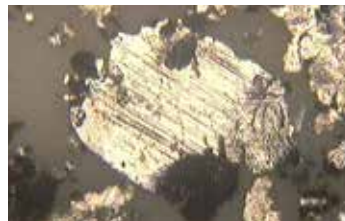
Particle with striation made from severe sliding
