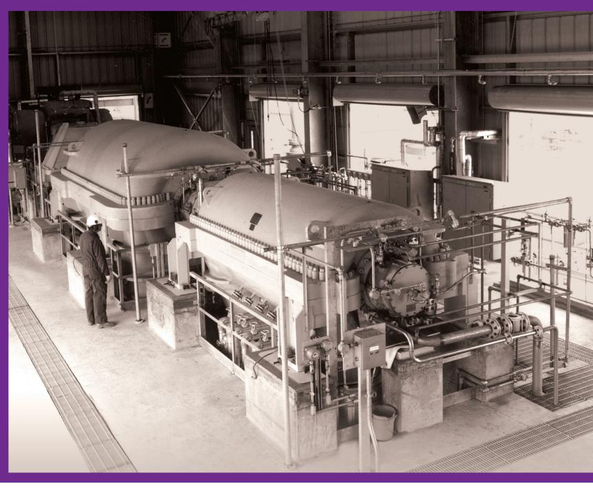
The power consumed by the compressor is proportional to the gas flow through the compressor. The key to compressor optimization is to deliver process needs with minimum possible flow through the compressor. In other words, minimize recycle or blow off.
