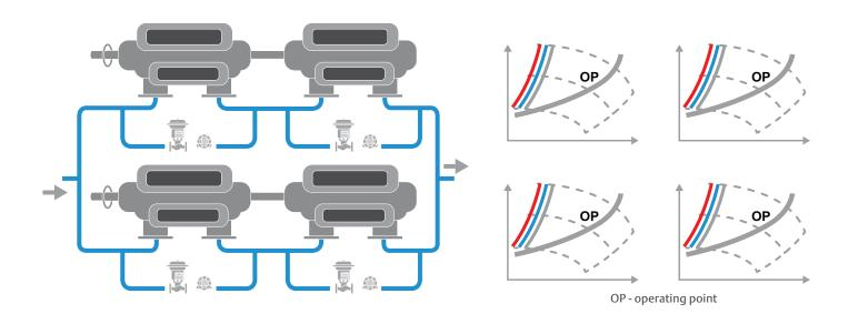
Optimizing efficiency: In case of parallel or series compressor operation, each compressor has its own unique compressor map as symbolically shown on the right.
