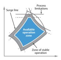
Advanced antisurge algorithms and control strategies allow the safe operating zone to be expanded. This helps decrease energy consumption when working close to the surge line and increases flexibility of the unit load.
