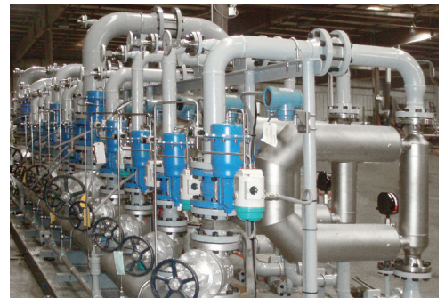
In-Line Fuel Blender used for Gasoline Blending at a Refinery.
