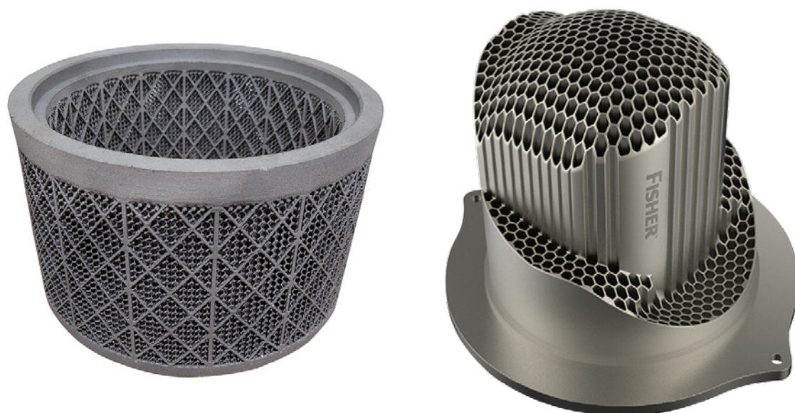
Figure 5. Additive manufacturing has made a whole new generation of innovative designs possible. Additively manufactured noise trim (left) controls valve noise with increased flow capacity, and the anti-cavitation trim (right) allows rotary valves to be installed and perform well in cavitating applications.
