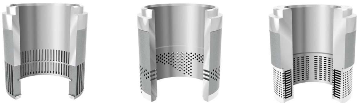
Figure 4. Low-noise trims vary from single-stage trim (left) to multipath (middle) to multipath and multistage (right). Higher pressure drops and vapor velocities typically require these types of complex trim designs.
