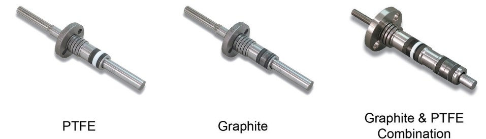
↑ Figure 3: Advanced environmental packing arrangements use carbon reinforced PTFE, graphite or combinations of reinforced PTFE and graphite rings to handle higher process temperatures and pressures, yet still achieve an emission rate less than 100 PPM.
