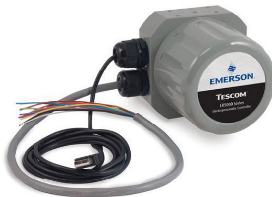
Figure 4. The ER5000 electropneumatic PID controller paired with a TESCOM regulator, both from Emerson, reduce exposure to hazardous gases with remote control without jeopardizing yield reliability. The ER5000 controller can be used as a stand-alone regulator or pilot regulator where precision and accuracy are critical to reach true repeatability. (Source: Emerson)
