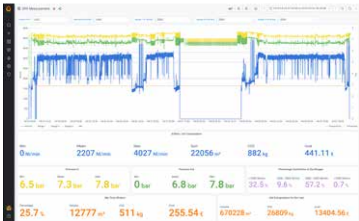
Live data captured by flow sensors using the AVENTICS Smart Pneumatics Analyzer. (Courtesy of Emerson)
