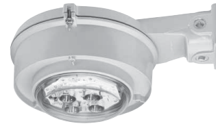
MERCMASTER™ LOW PROFILE LED LUMINAIRE NEC/CEC — CLASS I, DIVISION 2, GROUPS A, B, C, D; CLASS I, ZONE 2; TYPE 3R, 4X; IP66, IP67
