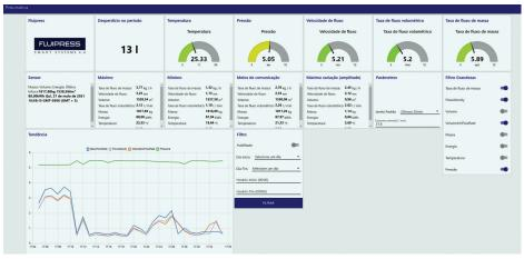
The AF2 flow sensor's calorimetric sensing cell measures air flow, pressure, velocity, volume, and energy. The device also calculates and stores descriptive statistics on the usage data.
