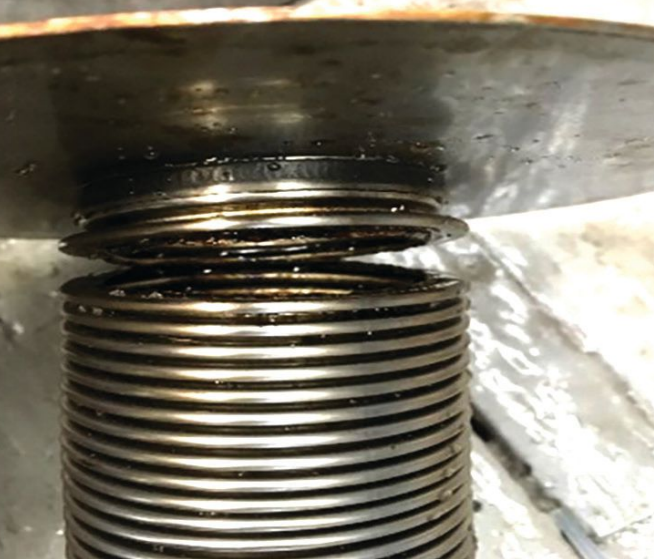
◀ Figure 3: Mechanical bellows are comparatively fragile and sensitive to metal fatigue and/or corrosive attack. A failed bellows leaks the process media to the environment and causes the PRV setpoint to vary with backpressure changes.
