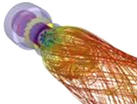
Figure 2 - CFD Depiction of the Turbulent Mixing of Fuel and Air Through a Burner
