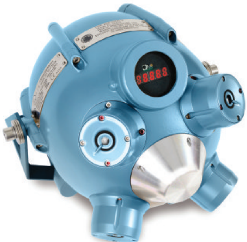
Figure 3 - Gas escaping under pressure produces an ultrasonic whistle in the range from 20 to 100 kHz that can be detected instantly at distances in excess of 10 metres, regardless of wind or weather
